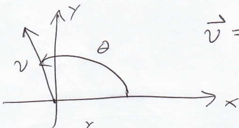
$$\vec{v} = \left( \underbrace{v \cos \theta}_{v_x}, \underbrace{v \sin \theta}_{v_y} \right)$$
