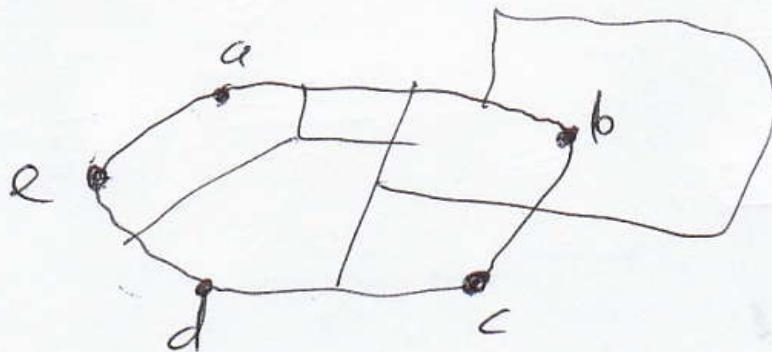
$$0 = V_{abcdea} = V_{ab} + V_{bc} + V_{cd} + V_{de} + V_{ea}$$
