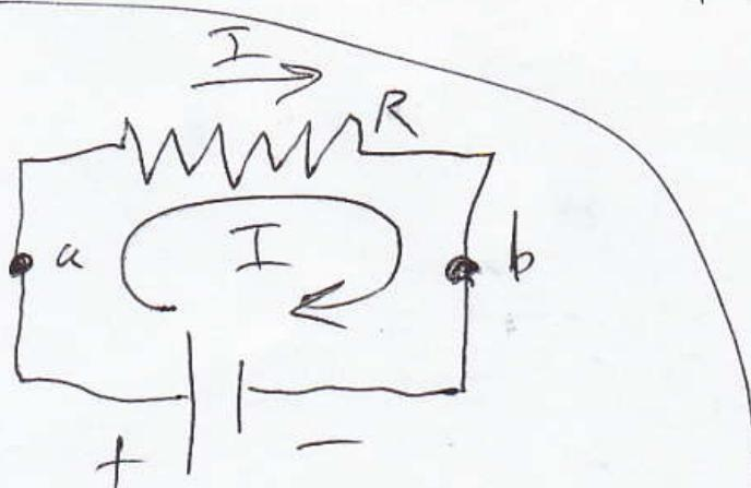
$$-V_{ba} = V_{ab} = IR$$
