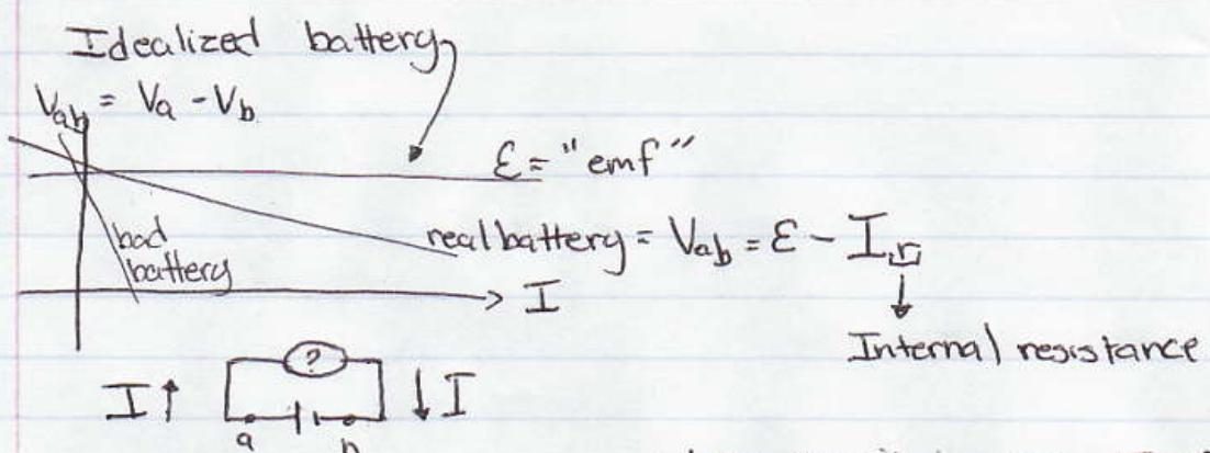
when circuit is open,  $I=0$ , so  $V_{ab}=E$
