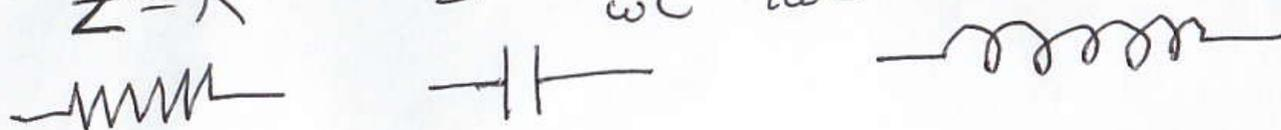
The diagram shows three circuit symbols: a resistor (zigzag line), a capacitor (two parallel lines), and an inductor (coiled line).
